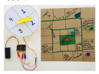
In this example, the servo is programmed to move to a random degree between 1 and 180 degrees. The number it turns to indicates the number of spaces to move on the hoard.
