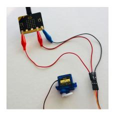
Once makers have successfully programmed a servo in the simulator and uploaded the code to the Micro:bit, it's time to connect the physical servo to the board. The Micro:bit should still be connected to the laptop.
