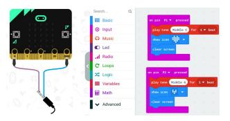
2. If you look closely at the cord from the speaker, you'll see 2 black stripes on the tip of the cable. On this audio plug, the bottom row is ground, and the middle and top of the cable are right and left audio.
