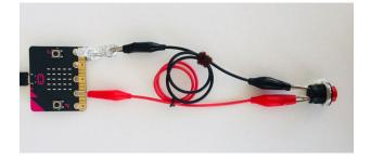
Repeat Steps 1 and 2 but connect to Pin 2 with a second button. You can connect to the aluminum foil on GND or connect to the metal alligator clip that's already on GND because the metal clip is conductive.
