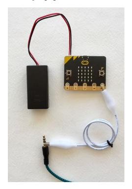
7. Next, connect an alligator clip from Pin 0 on the board to the top section of the 1/8" plug (left audio).
