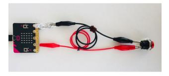
3. Repeat Steps 1 and 2 but connect to Pin 2 with a second button. You can connect to the aluminum foil on GND or connect to the metal alligator clip that's already on GND because the metal clip is conductive.
