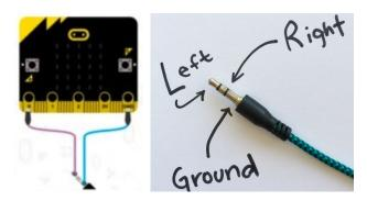
6. The bottom row is ground, so that will connect to **GND** on the Micro:bit. Connect an alligator clip from **GND** on the board to the lower section of the 1/8" pluq (ground).
