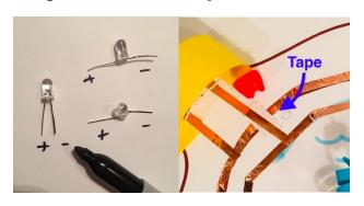
If lines of copper tape need to overlap, makers should insulate those sections by covering them with masking tape, creating a bridge so the copper lines don't touch. Two lines of copper tape touching (crossing of +/-) could cause a short circuit.
